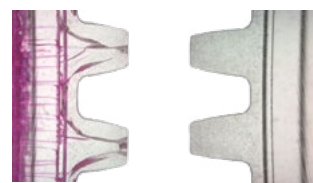
Stress cracked PC.
