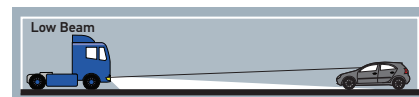
Designed to light the road at night without causing glare to other road users.
