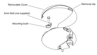
Clip the cover on securely until flush with the lamp surface.
